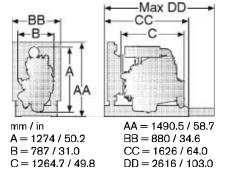
**Gen Pac** - Gen Set Engine mounted on an expandable base frame. Complete unit with engine, radiator, radiator core guard, fan, fan and belt guard providing reduced delivery time and inatallation cost and simplified transportation.
